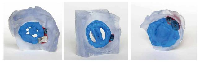
Figure 3. Printed PVL models with tested occluders
